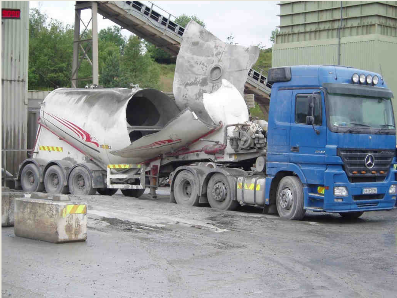
Failed Cement Tanker
